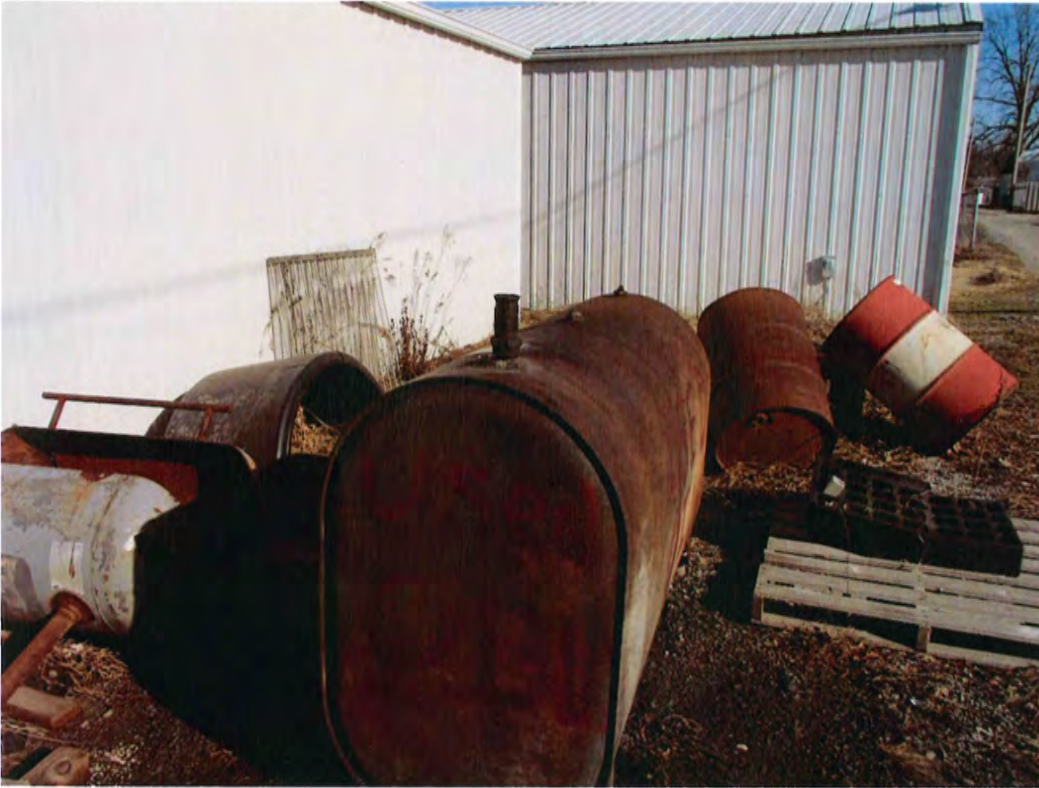
Date: 01/13/2014 Time: 1:28 P.M. Direction: east Photo by: Garrison Gross Exposure #: 005 Comments: used oil tank; bung not closed
